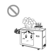
★Don't block the air intake or outlet vents of both the outdoor and indoor unit. It can decrease the air conditioning capacity or cause a malfunction.
